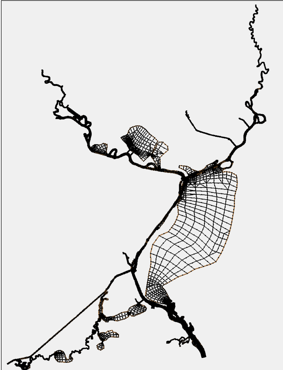
Figure 1 to Figure 3 show general details of a previously used numerical grid covering the SNWW. This grid was developed in support of a 2-D depth-averaged finite element RMA2 computational model, which over the years provided current data for various ship navigation simulation studies. These studies included the original deepening tests by the US Army
