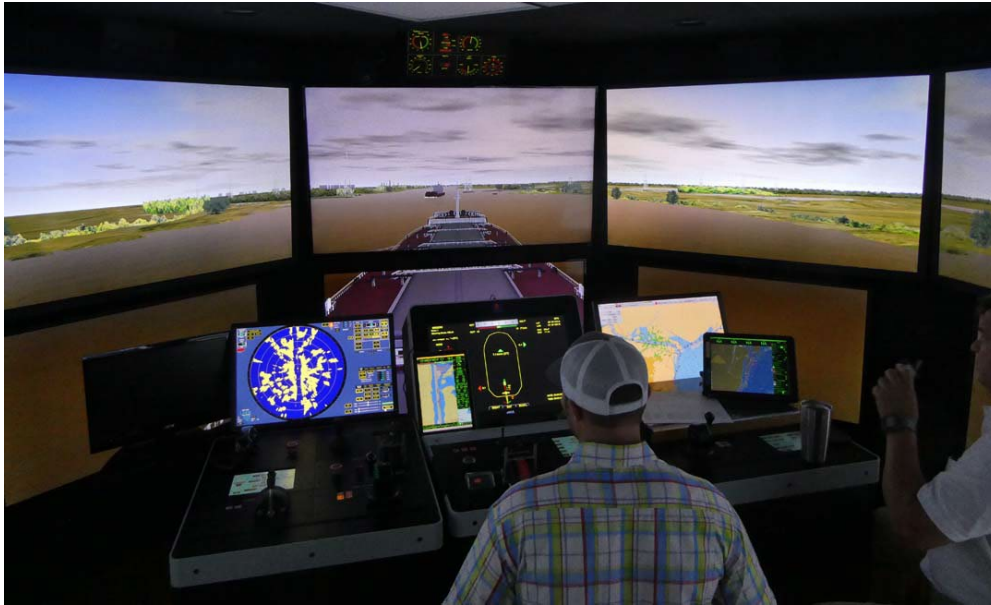
Figure 5. Sabine Pilot conning the MPI Full Mission Bridge Simulator
